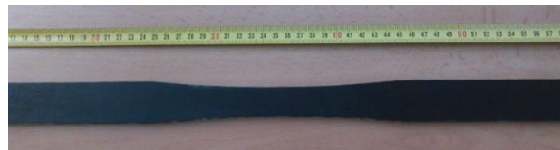
Fig. 2 Type A test specimen with marked gauge length
